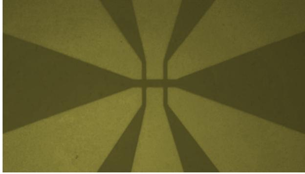
Figure 3.5: An optical image of completed Hall bar device.
